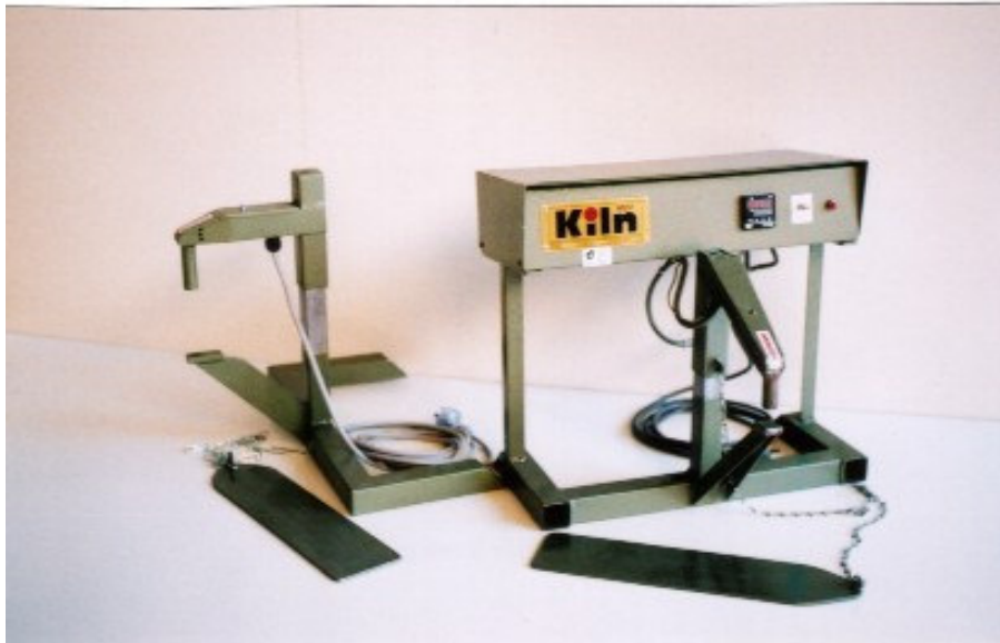
Photograph showing the master heater and a slave
